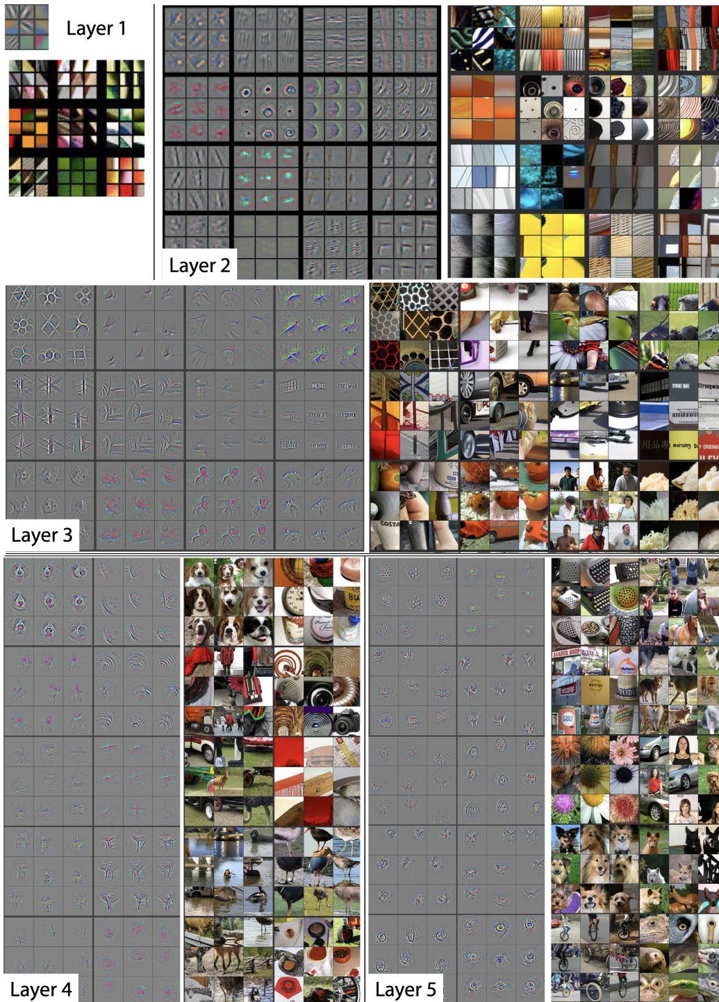
Figure 1.3: Visualization of features learned by a convolutional neural network. Early layers detect simple edges (top left), while deeper layers assemble these into complex geometries and object parts (middle, bottom). Note how these features naturally form a hierarchy of composition. Figure from Zeiler and Fergus [79].
